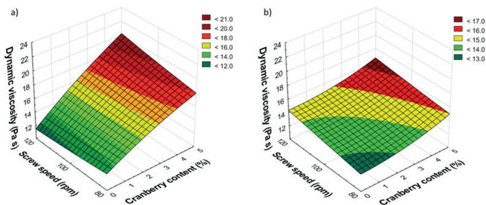
**Fig. 5.** Viscosity of 20% cold (a) and warm (b) suspension of corn grits with milk in relation to cranberry content and screw speed applied
