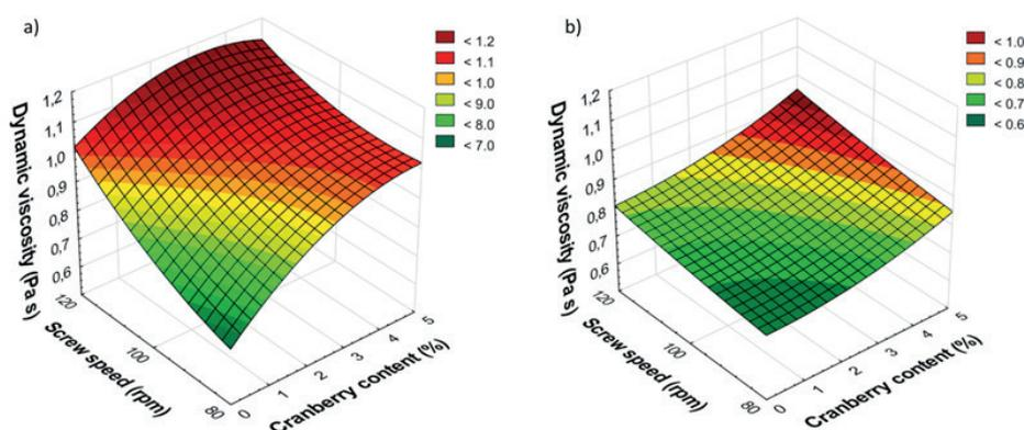
**Fig. 4.** Viscosity of 10% cold (a) and warm (b) suspension of corn grits with milk in relation to cranberry content and screw speed applied
