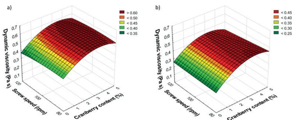
**Fig. 2.** Viscosity of 10% cold (a) and warm (b) suspension of extruded Gruels with water in relation to cranberry content and screw speed applied
