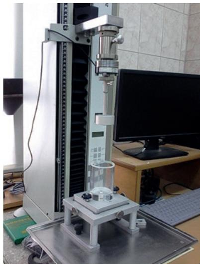
**Fig. 1.** Testing machine Zwick BDO-FB0.5TH with mounted “back-extrusion cell” device
