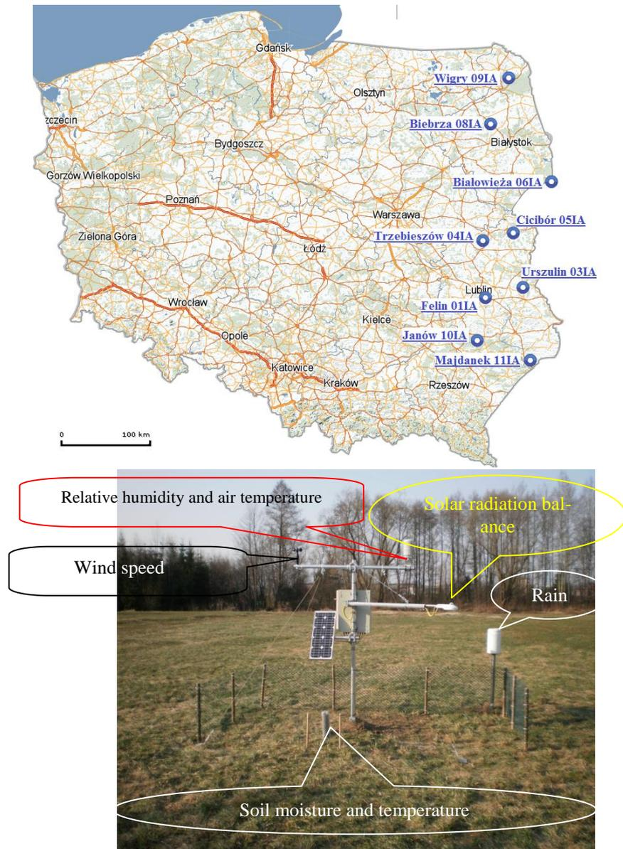
**Fig. 2.** Network of automatic agrometeorological stations (top panel) belonging to the Institute of Agrophysics in Lublin (background: Zumi Map (Zumi 2012)) and exemplary station in Janów (bottom panel)
