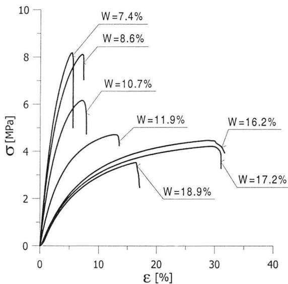
**Fig. 3.** Some of the strain-stress curves for the biodegradable plastic.
