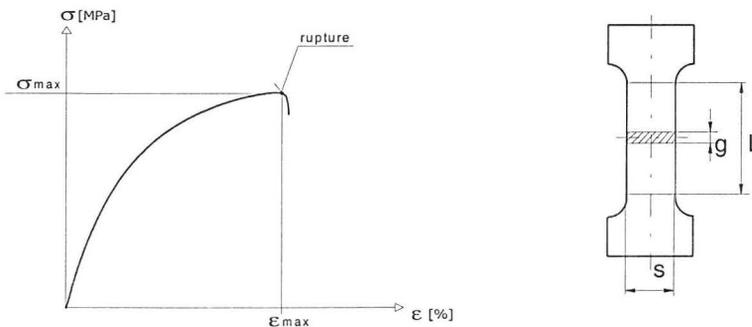
**Fig. 1.** Stress vs. strain curve of the biodegradable material.
