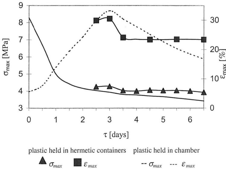
Fig. 6. Tensile strength properties of the plastic held in a climatic chamber and that moistened for 2.5 days and then held 4 days in hermetic containers.
