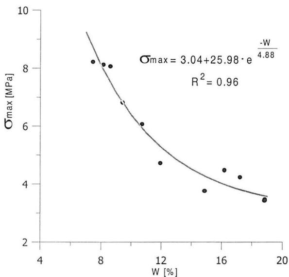
**Fig. 4.** Relation between breaking stress  $\sigma_{\max}$  and moisture content of the biodegradable material.
