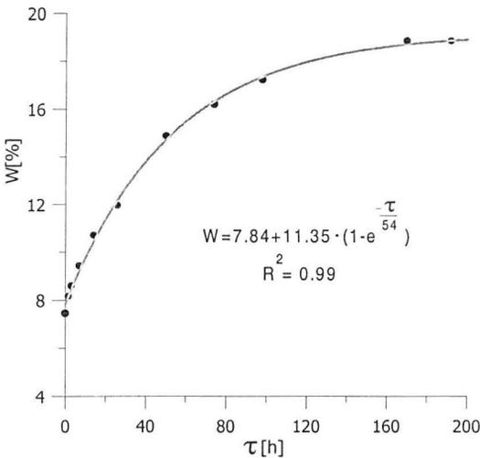
Fig. 2. Water absorption curve.
