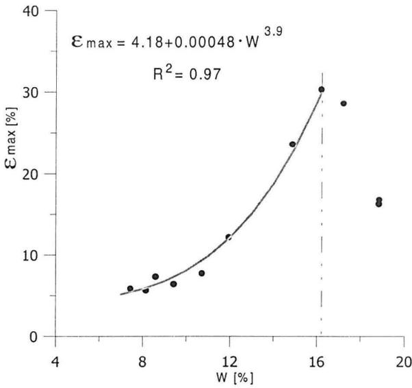
Fig. 5. Relation between the breaking strain  $\epsilon_{max}$  and moisture content of the biodegradable plastic.
