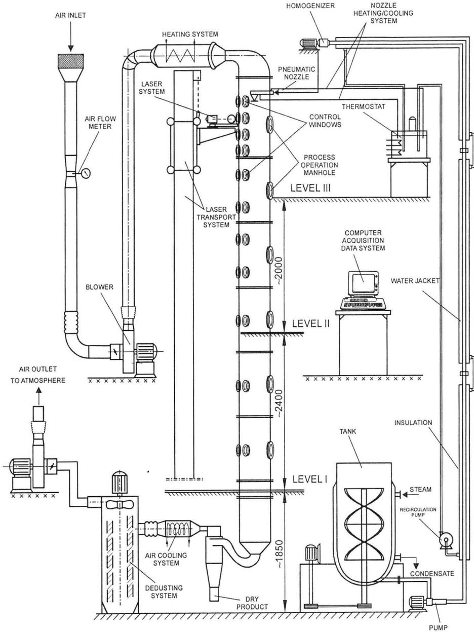
Fig. 1. Experimental set-up.
