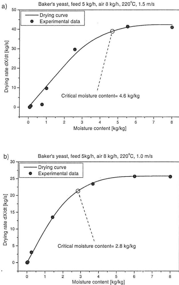
Fig. 5. Drying rate curves for different processes.
