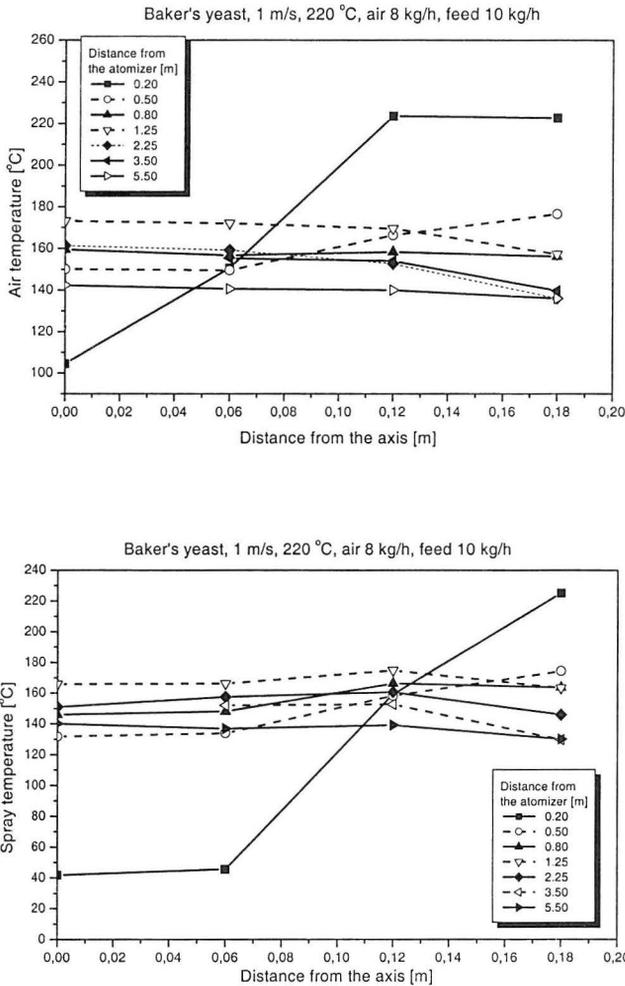
**Fig. 2.** Air and spray temperature distributions in the cross-sectional area of the spray tower (inlet temp. 220°C, atomizing air 8 kg/h, drying air velocity 1.0 m/s).
