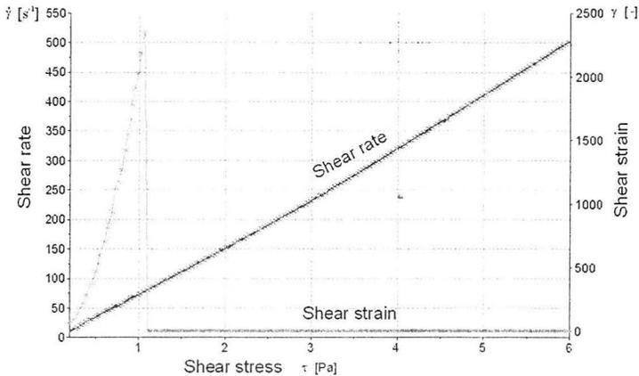
**Fig. 2.** Typical chart of shear rate  $\dot{\gamma}$  [s<sup>-1</sup>] and shear strain  $\gamma$  [-] in function of shear stress  $\tau$  [Pa] (product: liquid whole egg).
