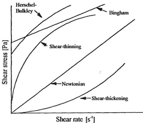
Fig. 1. Curves for typical time-independent fluids [10].
