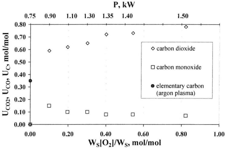
Fig. 4. The Freon decomposition degrees to  $CO_2$ ,  $CO$ , and  $C$  in relation to oxygen concentration in inlet gases and to input reactor power.
