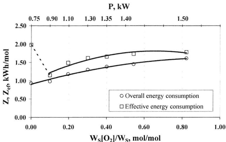
Fig. 6. The overall and effective energy consumption in relation to oxygen concentration in inlet gases and to input reactor power.
