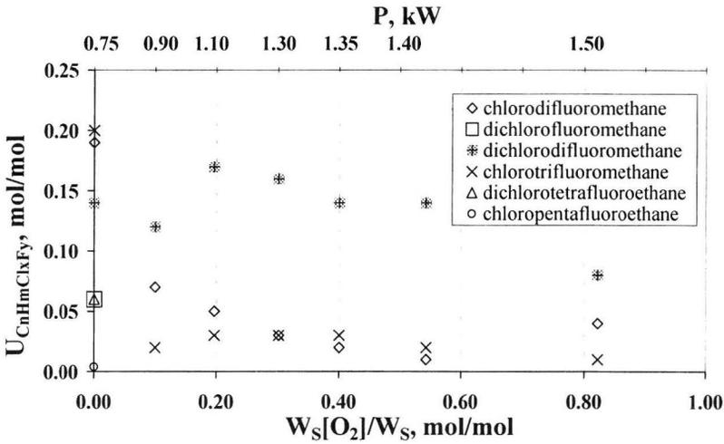
Fig. 5. The Freon decomposition degree to  $C_nH_mCl_xF_y$  in relation to oxygen concentration in inlet gases and to input reactor power.
