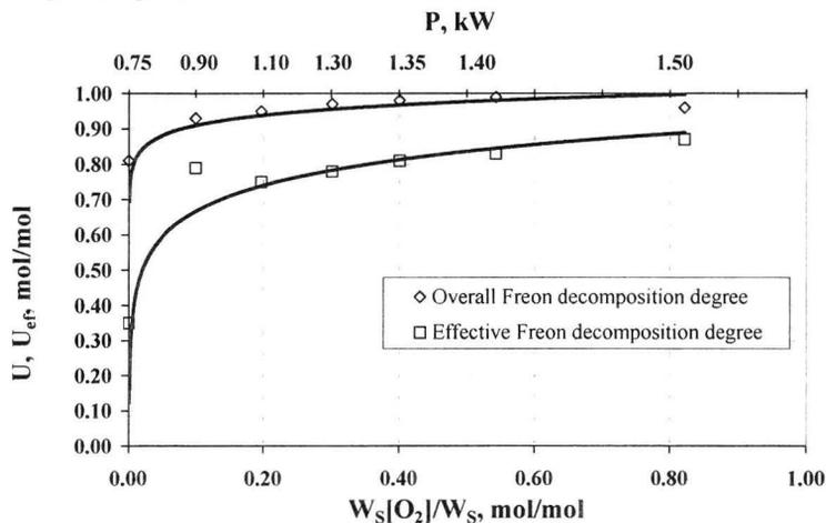
Fig. 3. The overall and the effective Freon decomposition degrees in relation to oxygen concentration in inlet gases and to input reactor power.
