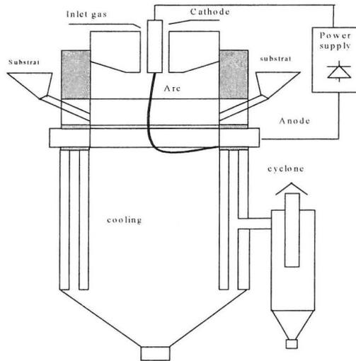
Fig. 3. DC rotating plasma system.
