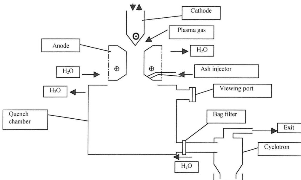
Fig. 2. DC plasma torch set-up.
