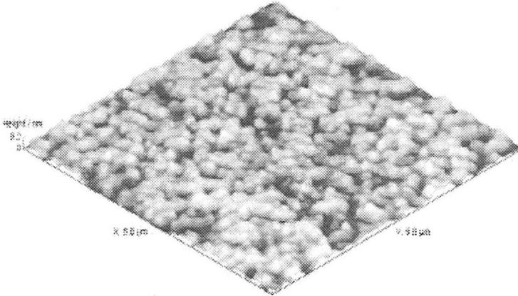
**Fig. 1.** Morphology of NCD layer observed by AFM method.
