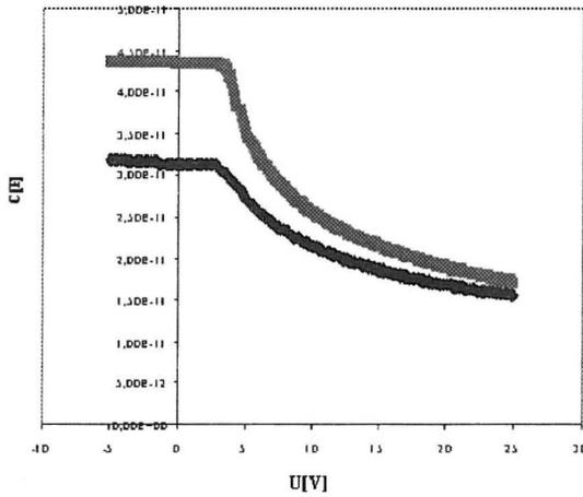
Fig.2. Typical change of electric properties of dielectric NCD layer in MIS ( AL/NCD/Si) structure.
