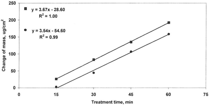
**Fig. 5.** Variation of the change of mass of PC plates with time of plasma treatment under process conditions of:
