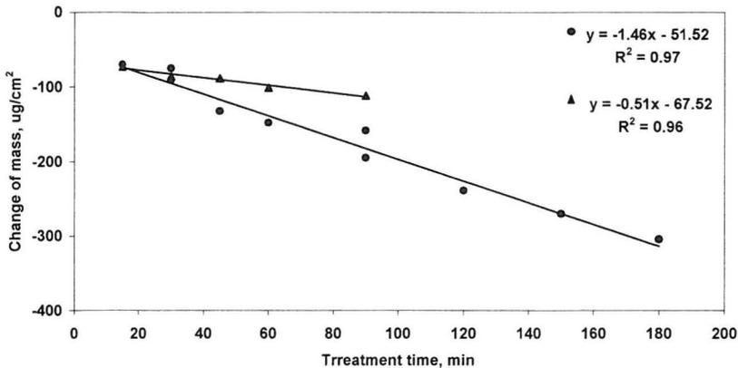
Fig. 4. Variation of change of mass of PC plates with time of plasma etching under process conditions of: PC plates placed at the high-voltage electrode, discharge gap - 0.75 mm, thickness of PC plates - 0.75 mm, discharge power - 0.25MW, ▲ - PC plates covered of thin film, ● - original PC plates.
