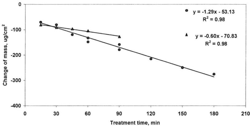
Fig. 3. Variation of change of mass of PC plates with time of plasma etching under process conditions of: PC plates placed at the grounded electrode, discharge gap - 0.75 mm, thickness of PC plates - 0.75 mm, discharge power - 0.25MW, ▲ - PC plates covered of thin film, ● - original PC plates.
