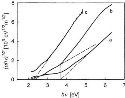
**Fig. 2.** Optical absorption edges presented according to the Tauc relation for a-Si<sub>x</sub>C<sub>y</sub>:H films deposited at various  $V_{(-)}$ : (a) 100 V; (b) 500 V; (c) 1100 V.
