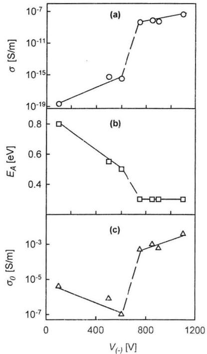
**Fig. 1.** Electrical conductivity of a-Si<sub>x</sub>C<sub>y</sub>:H films as a function of  $V_{(-)}$ : (a) specific conductivity; (b) activation energy; (c) pre-exponential factor.
