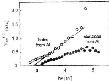
**Fig. 5.** Fowler's diagram for the  $a\text{-Si}_x\text{C}_y\text{:H}$  semiconducting films.
