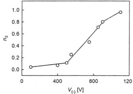
**Fig. 3.** Semiconducting fraction content  $n_s$  in the a-Si<sub>x</sub>C<sub>y</sub>:H films as a function of  $V_{(-)}$ .
