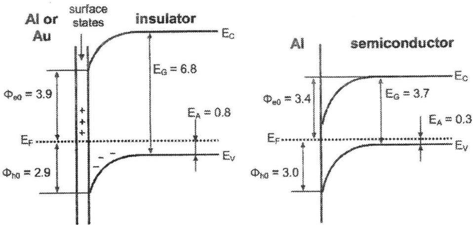
Fig. 6. Band structure models for insulating and semiconducting a-Si<sub>x</sub>C<sub>y</sub>:H films in the region of the film-metal contacts. All values are given in eV.
