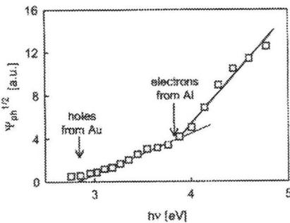
**Fig. 4.** Fowler's diagram for the  $a\text{-Si}_x\text{C}_y\text{:H}$  insulating films.
