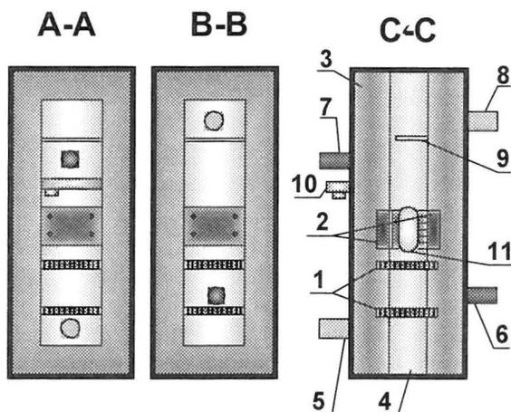
Fig. 1. Foaming column. (1-diffusers, 2-electrodes, 3-housing, 4-spacer, 5-gas inlet, 6-liquid inlet, 7-liquid outlet, 8-gas outlet, 9-drops' grabber).
