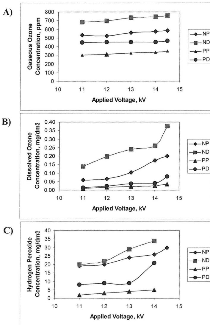
**Figs. 3.** The comparison of the oxidants concentrations obtained in the foaming system in dependence on applied voltage at constant  $8 \text{ dm}^3 \text{ min}^{-1}$  oxygen flow rate. A) gaseous ozone, B) dissolved ozone, C) hydrogen peroxide.
