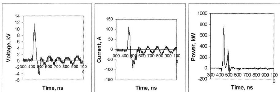
**Figs. 2.** Electrical characteristics and absolute power of the discharges in needle-to-metal plate electrode set-ups. Airflow rate: 8 l/min. 14 kV of applied voltage.
