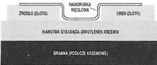
Fig. 5. FET transistor with silicon substrate as gate; acc. to [3].
