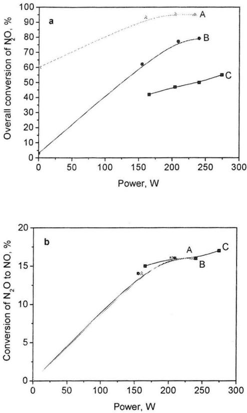
**Fig. 3.** Effect of discharge power on overall conversion of nitrous oxide (a) and conversion of nitrous oxide to NO (b). Interelectrode gape width 1 mm, initial nitrous oxide concentration 5% by vol. Nozzle with inner diameter 1.75mm. A - reactor without catalyst. B - reactor with catalyst ( $T=480^\circ\text{C}$ ), C - reactor with catalyst ( $T=600^\circ\text{C}$ ).
