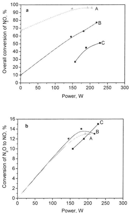
**Fig. 4.** Effect of discharge power on overall conversion of nitrous oxide (a) and conversion of nitrous oxide to NO (b). Interelectrode gap width 1 mm, initial nitrous oxide concentration 5% by vol. Nozzle with inner diameter 0.75mm. Reactor with modified reaction space. A - reactor without catalyst, B - reactor with catalyst ( $T=480^{\circ}\text{C}$ ), C - reactor with catalyst ( $T=600^{\circ}\text{C}$ ).
