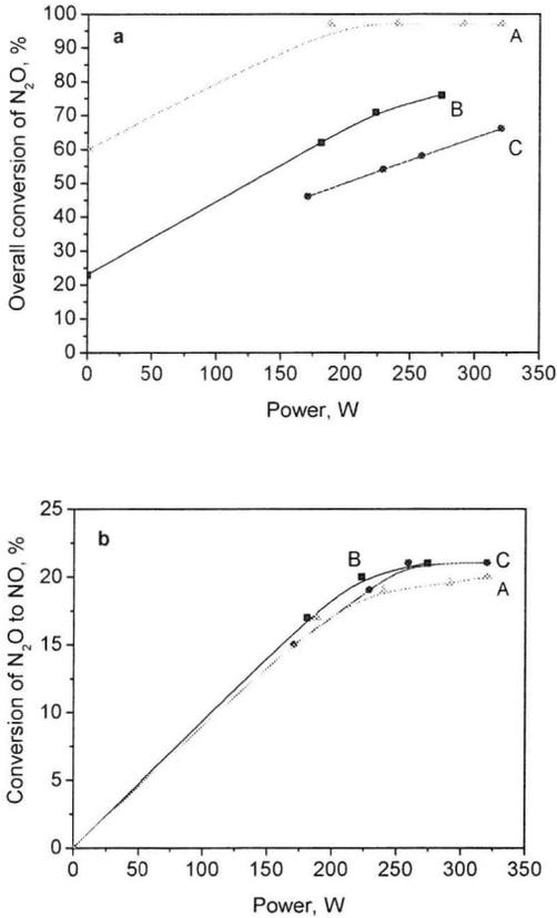
**Fig. 2.** Effect of discharge power on overall conversion of nitrous oxide (a) and conversion of nitrous oxide to NO (b). Interelectrode gape width 1 mm, initial nitrous oxide concentration 5% by vol. Nozzle with inner diameter 0.75mm. A - reactor without catalyst, B - reactor with catalyst ( $T=480^\circ C$ ), C - reactor with catalyst ( $T=600^\circ C$ ).
