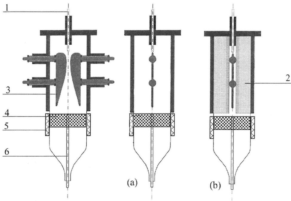
**Fig.1.** Reactors for nitrous oxide conversion: (a) - unmodified reactor, (b) – reactor after modification. 1 – gas inlet nozzle, 2 – ceramic filling, 3 - electrodes, 4 – packing bed, 5 – heating jacket, 6 – thermocouple.
