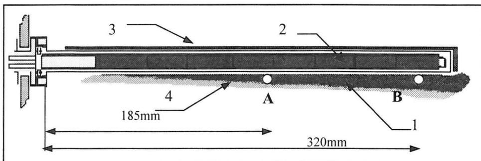
**Fig. 1.** The cathode of the linear magnetron and positions of OES measurement. (1) plasma zone; (2) magnetic system; (3) shield; (4) cathode (target); (A), (B) optical viewpoints.
