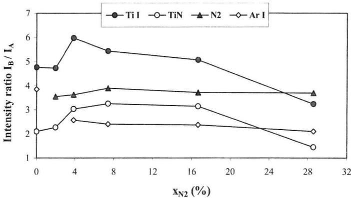
Fig. 4. Intensity ratios for spectra obtained from viewports A and B versus nitrogen amount in the Ar+N<sub>2</sub> mixture.
