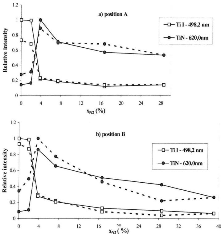
**Fig. 2.** Variations of Ti I and TiN intensities in position A (a) and B (b) with increasing (solid line) and decreasing (dotted line) nitrogen content in the Ar+N<sub>2</sub> mixture. Intensities are normalized to 1 at the maximum value.
