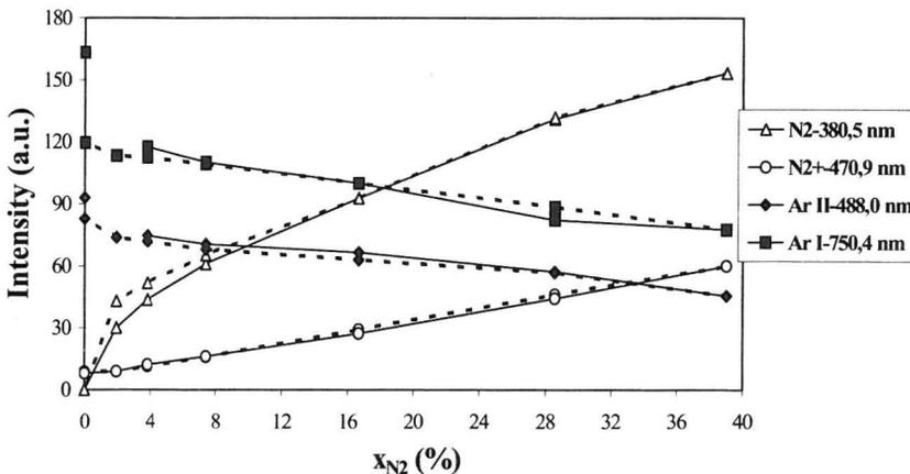
Fig. 3. Changes in emission intensities of argon and nitrogen species with increasing (solid line) and decreasing (dotted line) nitrogen content in the Ar+N<sub>2</sub> mixture. The results for the position B.
