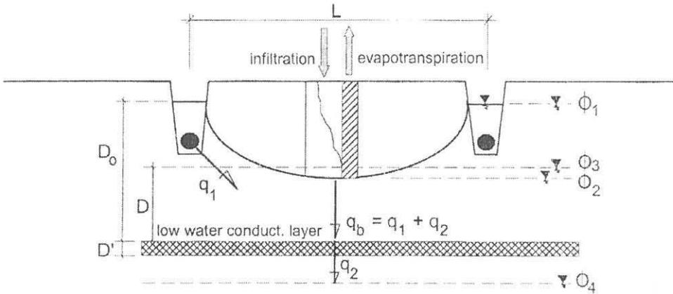
Fig. 1. Physical concept of the SWATREZ model
