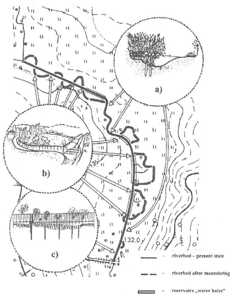
Fig. 1. The Rudnia's river valley segment of intend for restoration, technical activities proposed: a) riverbed narrowing structures, b) dykes affecting water flow by meanders, c) stone spillway
