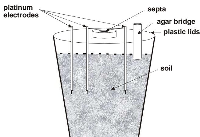
Fig. 1. Schematic of the incubation containers
