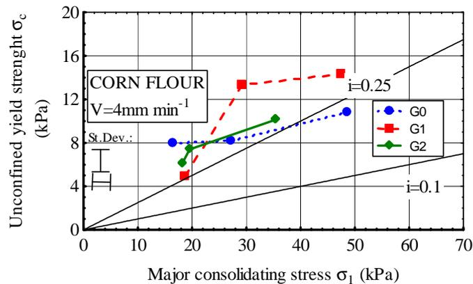
Fig. 6. Mean values of flow functions of corn flour for 4 mm min<sup>-1</sup> speed of deformation
