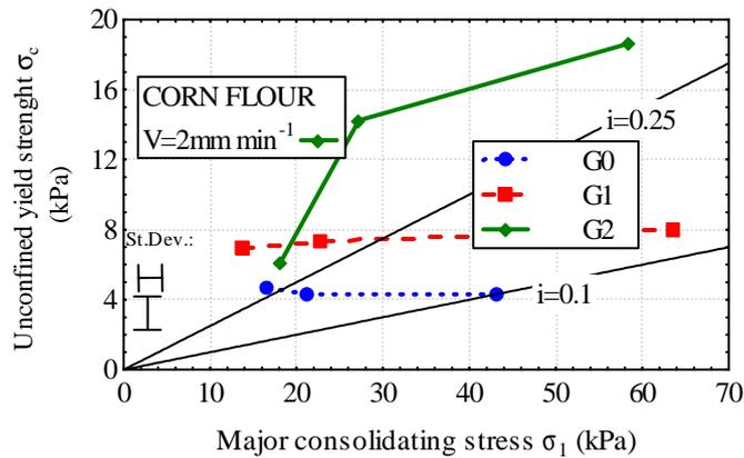
Fig. 5. Mean values of flow functions of corn flour for 2 mm min<sup>-1</sup> speed of deformation
