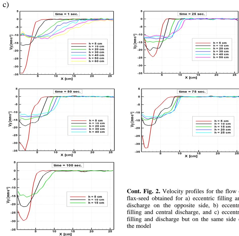
**Cont. Fig. 2.** Velocity profiles for the flow of flax-seed obtained for a) eccentric filling and discharge on the opposite side, b) eccentric filling and central discharge, and c) eccentric filling and discharge but on the same side of the model
