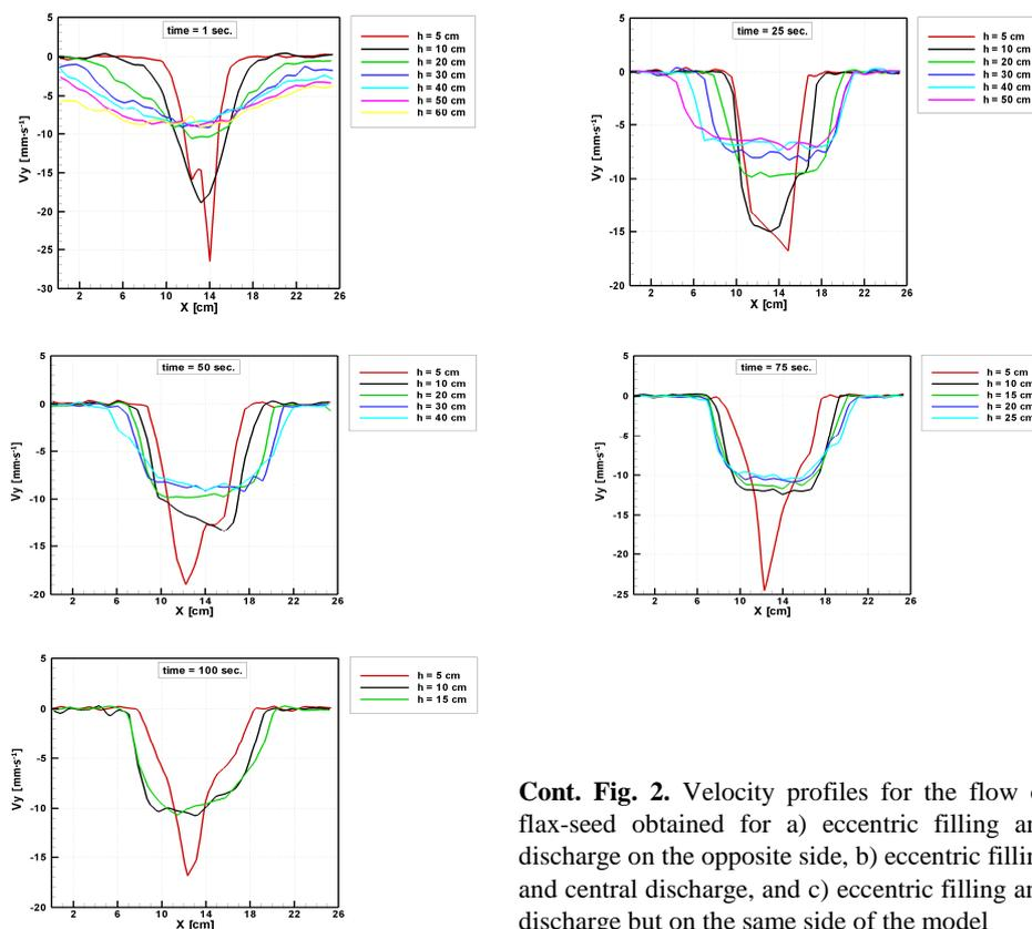
**Cont. Fig. 2.** Velocity profiles for the flow of flax-seed obtained for a) eccentric filling and discharge on the opposite side, b) eccentric filling and central discharge, and c) eccentric filling and discharge but on the same side of the model
