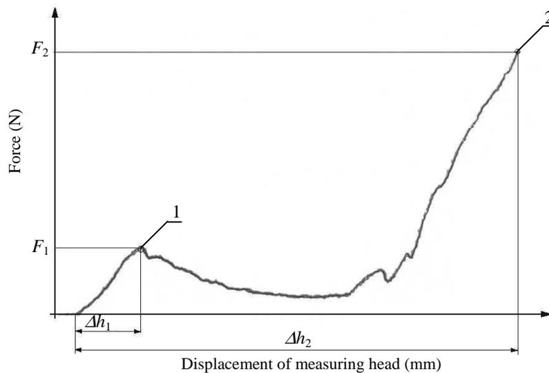
**Fig. 1.** Example of wheat kernel compression curve. 1 – rupture point, 2 – the end of compression
