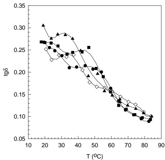
**Fig. 2.** Temperature dependencies of the loss tangent for the batter samples with fat replaced by starch preparation in three forms: dry mass - square points, suspension - triangle points, gel - diamond points) and for the control sample - circle points
