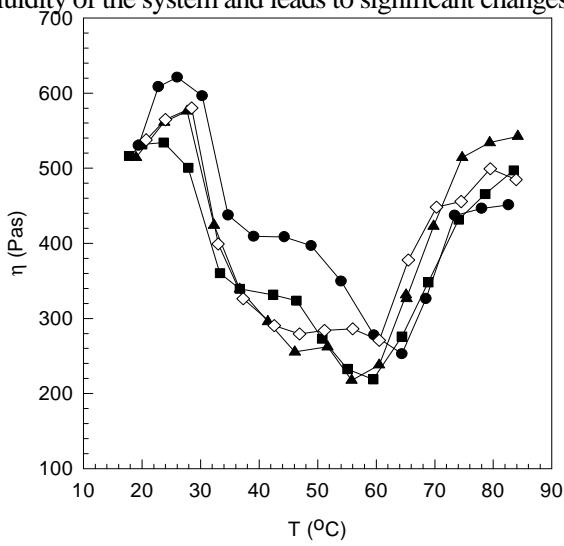
**Fig. 3.** Temperature dependencies of the dynamic viscosity for the batter samples with fat replaced by starch preparation in three forms: dry mass – square points, suspension – square points, gel – diamond points) and for the control sample – circle points
