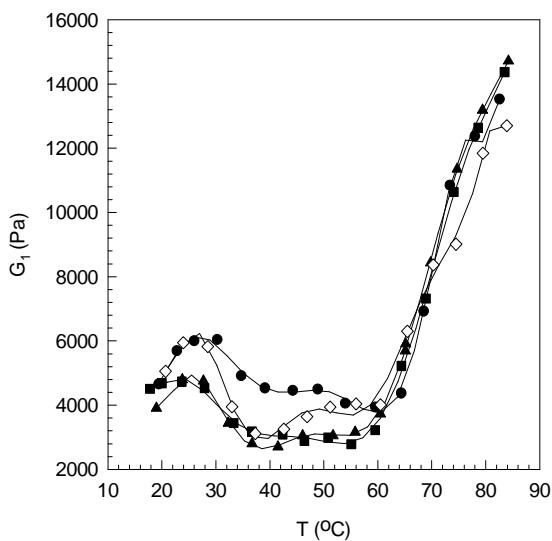
**Fig. 1.** Temperature dependencies of the real component of the elasticity modulus ( $G_I$ ) for the batter samples with fat replaced by starch preparation in three forms: dry mass - square points, suspension - triangle points, gel - diamond points) and for the control sample - circle points
