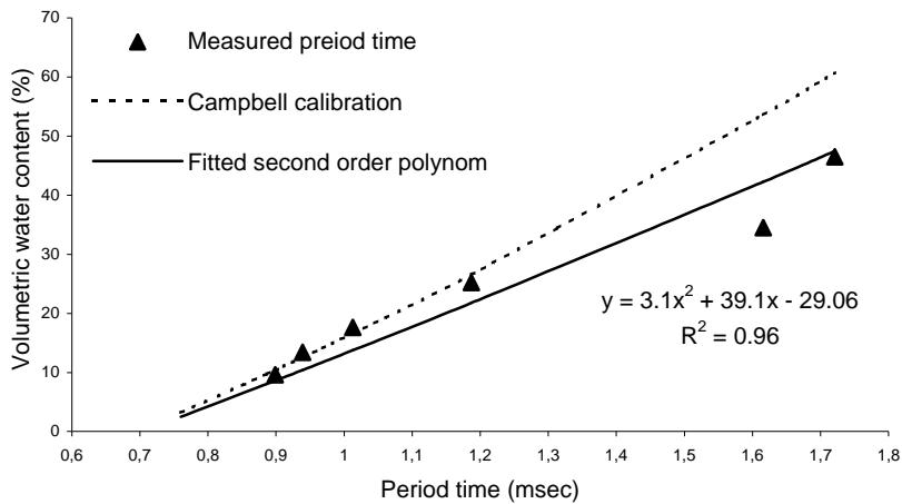
**Fig. 5.** The CS615 sensor calibration curve for the soil of the beech forest study site
