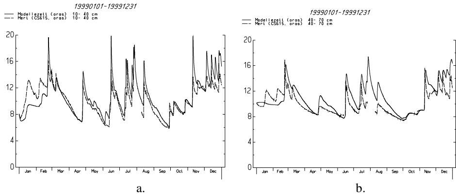
**Fig. 4.** The measured TDR and simulated soil water content time dynamics of the 10-40 cm (a) and 40-70 (b) cm soil layers
