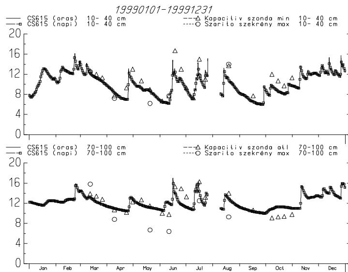
**Fig. 2.** CS615 (—), BR-150 ( $\Delta$ ) and oven dried (o) soil water content data of the Scotch pine stand
