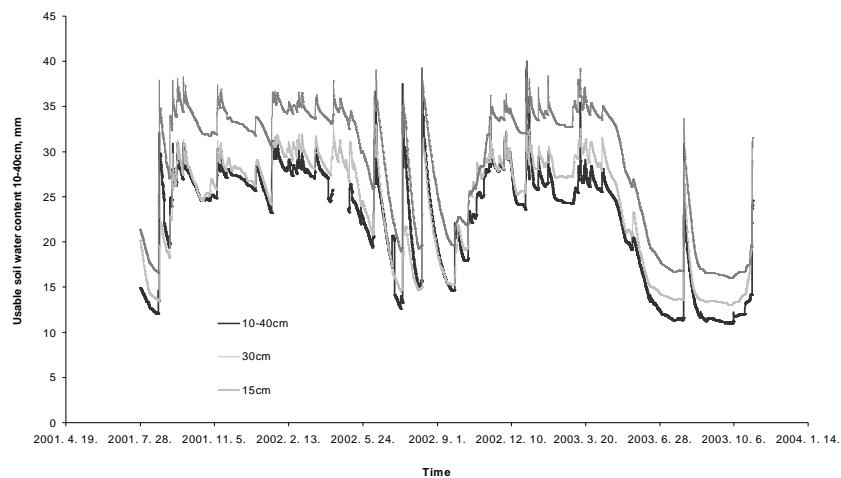
**Fig. 6.** The CS615 recorded soil water content dynamics in the soil of the beech forest study site
