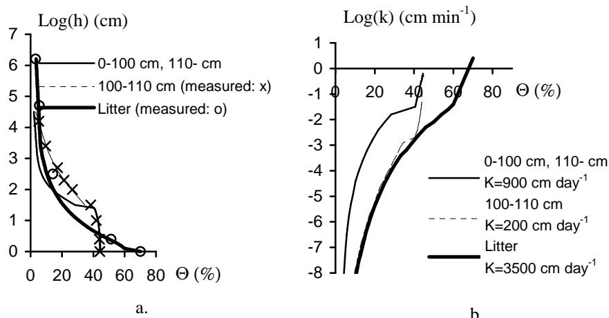
**Fig. 1.** The water retention (a) and water conductivity (b) data and functions of the lowland sandy soil and litter. The 100-110 cm depth is a buried humus layer in the soil profile
