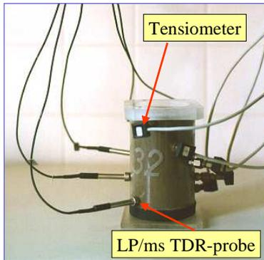
**Fig. 1.** Equipment for simultaneous measurement of soil water potential and soil moisture
