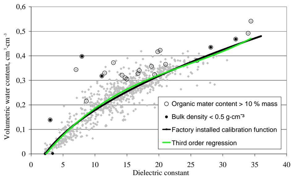
**Fig. 3.** Measurements compared with the factory installed calibration function concerning the dielectric constant and the water content of the
