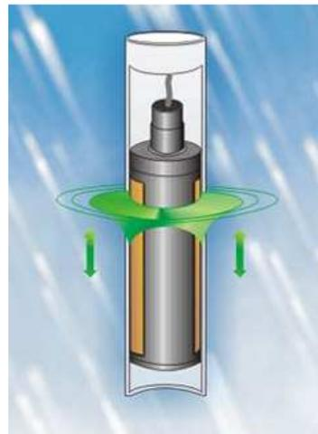
**Fig. 4.** Schematic view of the Trime<sup>®</sup> Tube Probe with indication of its electromagnetic field
