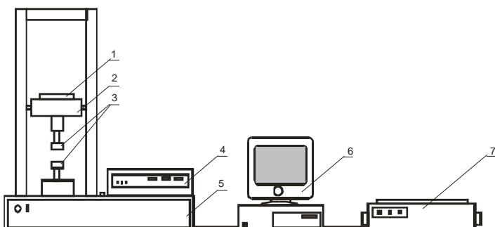
**Fig. 2.** Schematic of a laboratory stand for testing the process of juice pressing: 1 – upper mobile head, 2 – Instron testing machine, 3 – laboratory press, 4 – control desk, 5 – lower stationary machine table, 6 – monitor, 7 – printer
