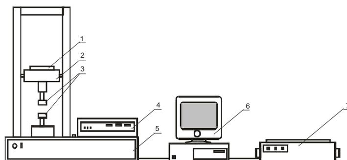
Fig. 2. Schematic of a laboratory stand for testing the process of juice pressing: 1– upper mobile head, 2 – Instron testing machine, 3 – laboratory press, 4 – control desk, 5 – lower stationary machine table, 6 – monitor, 7 – printer
