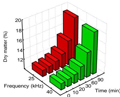
**Fig. 5.** Dry matter content as a function of frequency and time of sonication for grape variety Portugalskie Niebieskie
