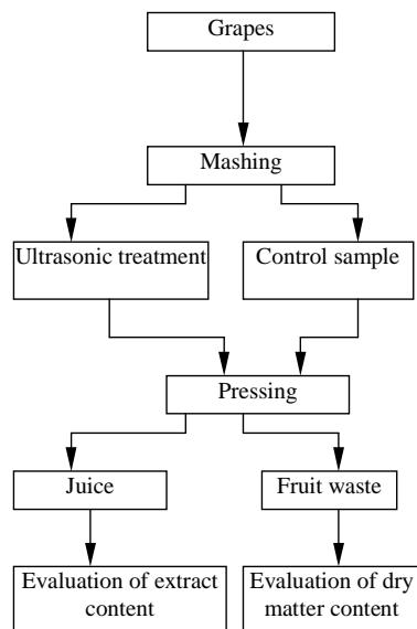
**Fig. 1.** Flow diagram of juice grape pressing
