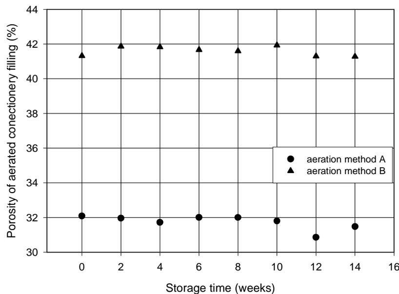
Fig. 2. Effect of storage time on porosity of confectionery filling obtained by two methods of aeration
