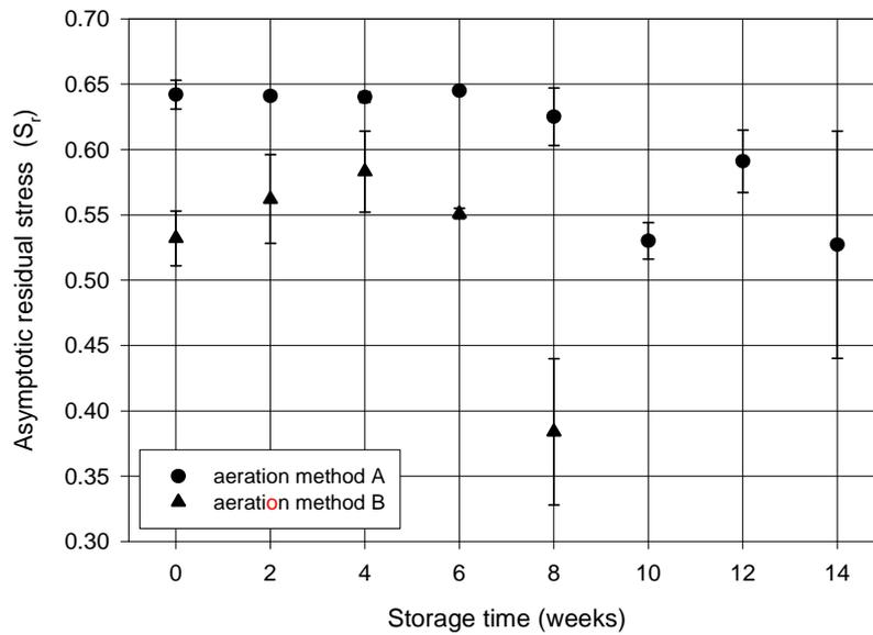
**Fig. 6.** Effect of storage time on asymptotic residual stress of confectionery filling obtained by two methods of aeration
