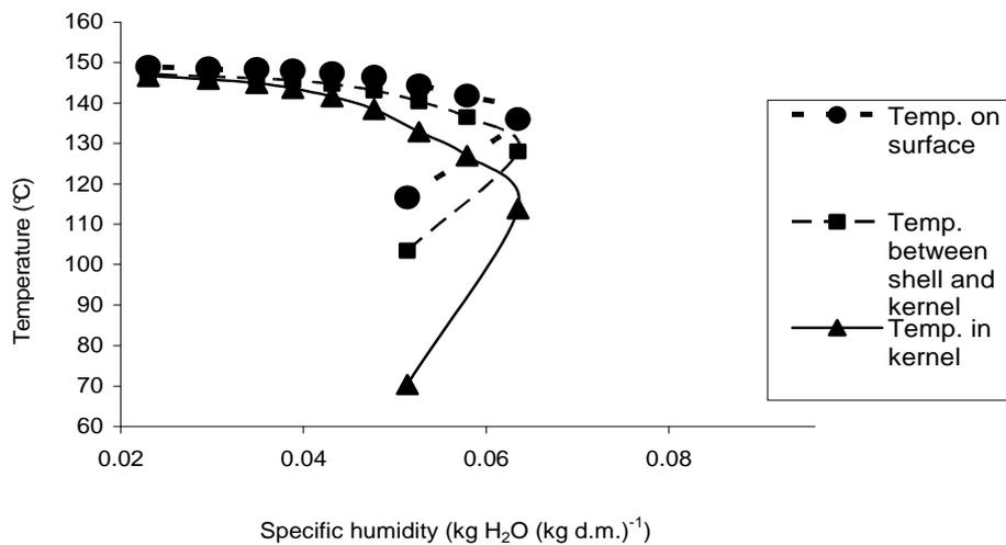
**Fig. 7.** Changes in temperature of selected parts of cocoa bean roasted for 20 min at 150°C (air flow rate of 1 m s<sup>-1</sup> and relative air humidity of 5%).
