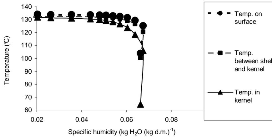
**Fig. 6.** Changes in temperature of selected parts of cocoa bean roasted for 50 min at 135°C (air flow rate of 1 m s<sup>-1</sup> and relative air humidity of 5%)
