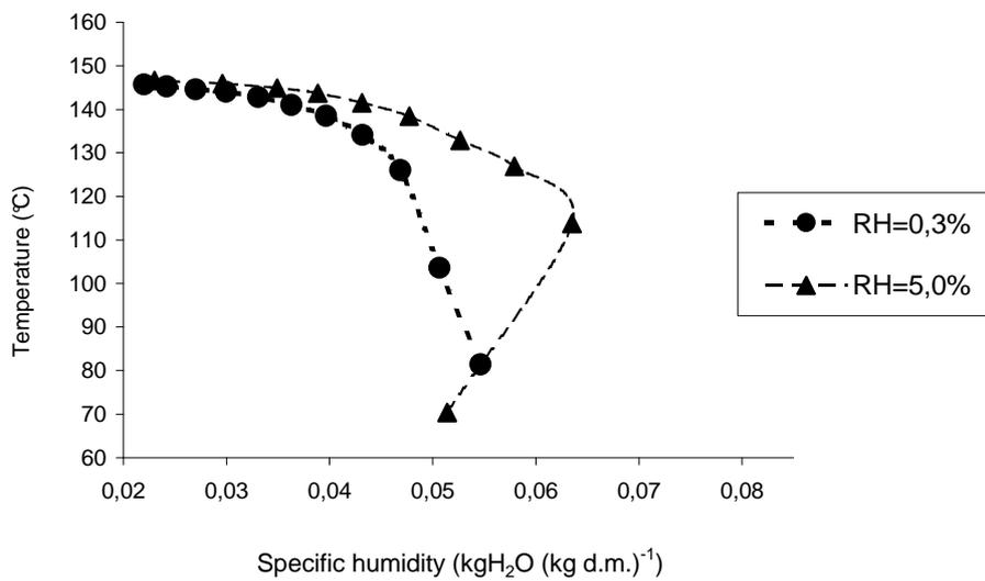
**Fig. 9.** Changes in temperature in the kernel in cocoa beans roasted at  $T = 150^{\circ}\text{C}$ ;  $v = 1 \text{ m s}^{-1}$
