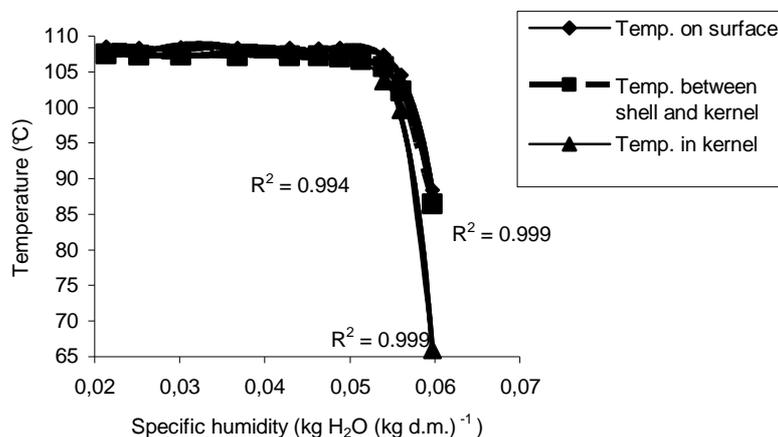
**Fig. 2.** Changes in temperature of selected parts of cocoa bean roasted for 70 min at 110°C (air flow rate of 1 m s<sup>-1</sup> and relative air humidity of 0.9%)
