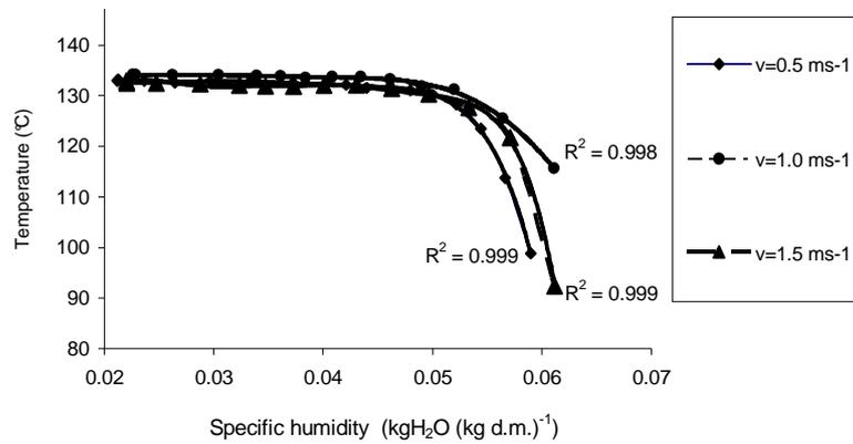
**Fig. 4.** Changes in temperature between the kernel and shell in cocoa beans roasted at  $T = 135^{\circ}\text{C}$ ;  $RH = 0.4\%$
