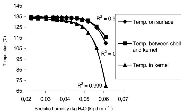
**Fig. 3.** Changes in temperature of selected parts of cocoa beans roasted for 35 min at 135°C (air flow rate of 1 m s<sup>-1</sup> and relative air humidity of 0.4%).
