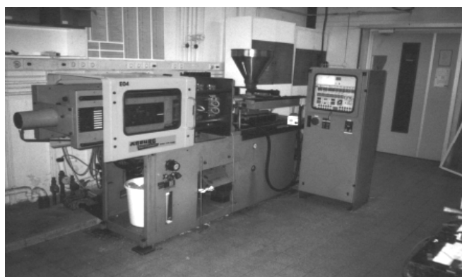
Fot. 4. Wtryskarka ARBURG 220H90-350 Photo 4. Injection moulding machine ARBURG 220H90-350
