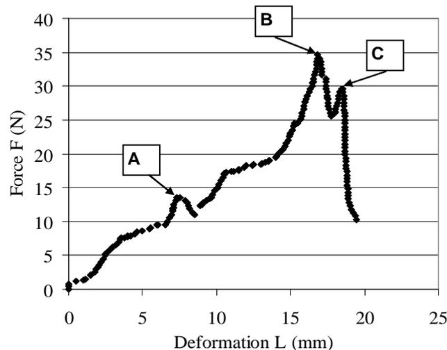
Fig. 1. Example of the course of the carrot cutting process
