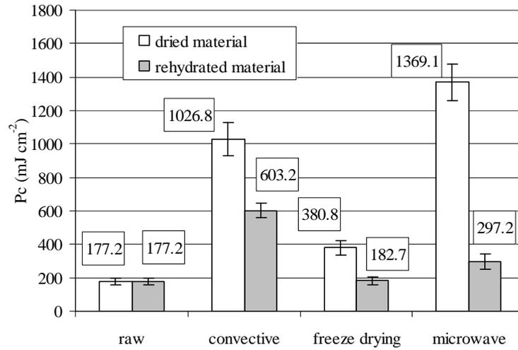
**Fig. 3.** Values of the total cutting work for carrot dehydrated osmotically before drying
