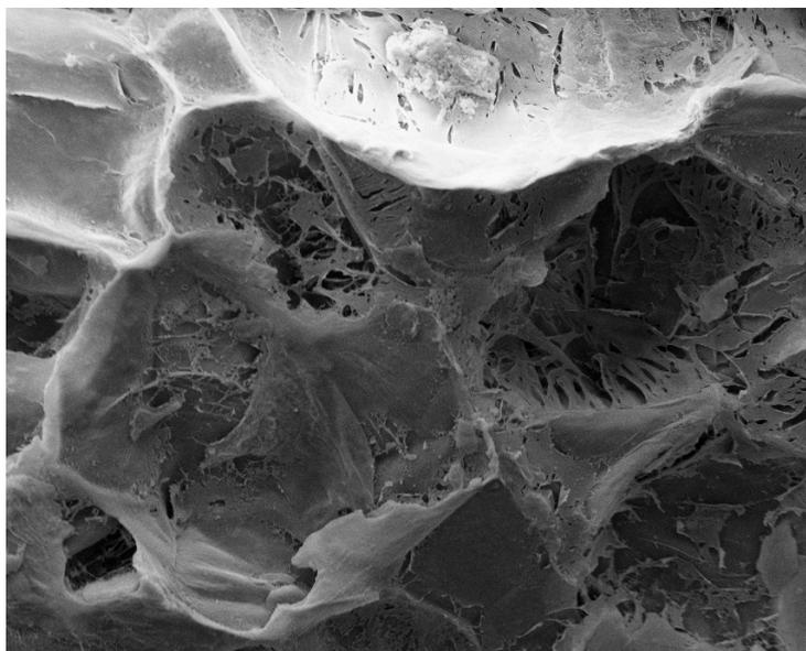
**Photo. 3.** Photograph of hydrated carrot material, blanching, and sublimation dried (magnification 700x)
