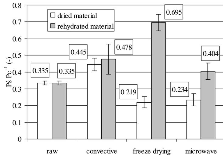
**Fig. 4.** Values of the compression degree of carrot cut and blanched before drying
