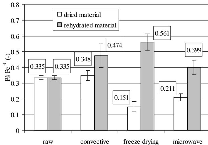
**Fig. 5.** Values of the compression degree of carrot cut and dehydrated osmotically before drying
