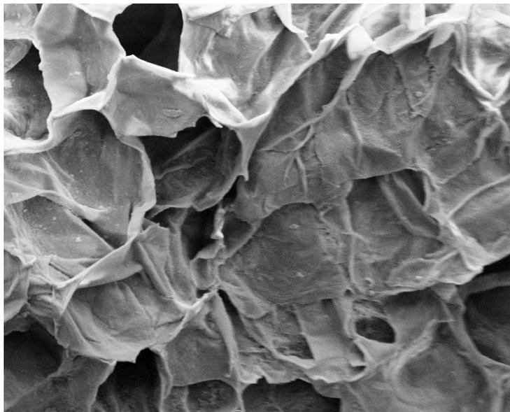
**Photo. 5.** Photograph of hydrated carrot material, blanching, and sublimation dried (magnification 700x)
