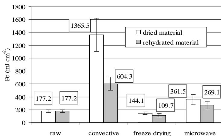
**Fig. 2.** Values of the total cutting work for carrot blanched before drying
