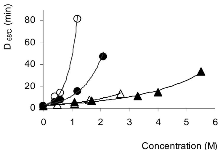
**Fig. 5.** Decimal reduction time  $D$  for  $\alpha$ -amylase isothermal inactivation at  $68^\circ\text{C}$  in correlation with the concentration of sorbitol ( $\Delta$ ), glycerol ( $\blacktriangle$ ), trehalose ( $\bullet$ ), sucrose ( $\circ$ )
