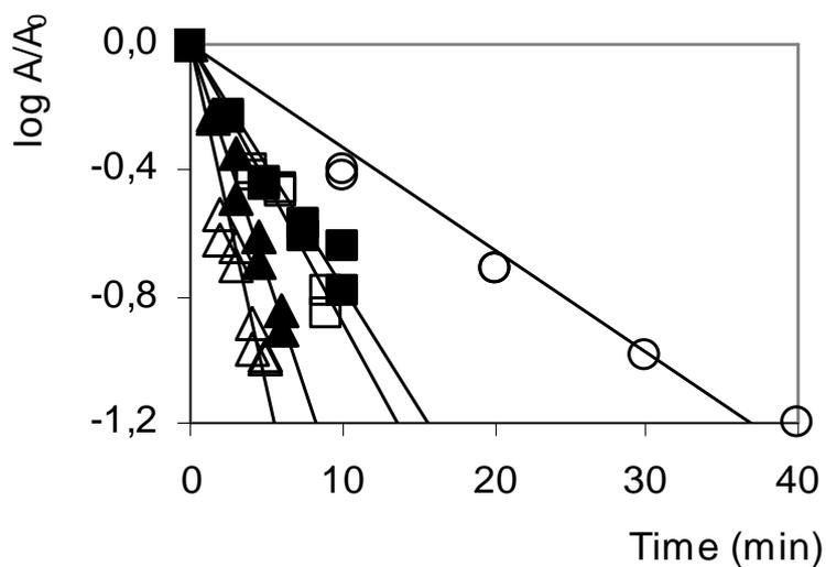
**Fig. 2.** Isothermal inactivation of  $\alpha$ -amylase in 20 mM Bis-Tris buffer, pH 7.0, with addition of glycerol: 8,3 % v/v ( $\Delta$ ), 13 % v/v ( $\blacktriangle$ ), 24,8 % v/v ( $\square$ ), 30 % v/v ( $\blacksquare$ ), 41 % v/v ( $\circ$ )
