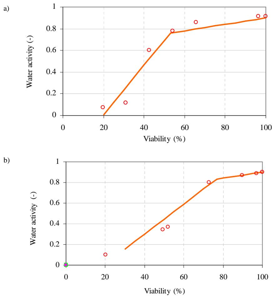
**Fig. 1.** Viability of yeast *Saccharomyces cerevisiae* freeze-dried without addition of lactose (a) and with lactose (b) as a function of water activity
