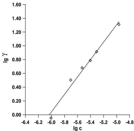
**Fig. 5.** Linear relationship between  $\gamma = \lg(F_0 - F)/(F - F_\infty)$  and the  $\lg c$ , where  $c$  is ferriCY concentration in  $\mu\text{M}$ . Relative fluorescence intensities ( $F$ ) at 645 nm,  $F_0$  – without ferriCY (20.0  $\mu\text{M}$ ),  $F_\infty$  – saturation value. Excitation wavelength 425 nm. FerriCY concentration 1-11  $\mu\text{M}$
