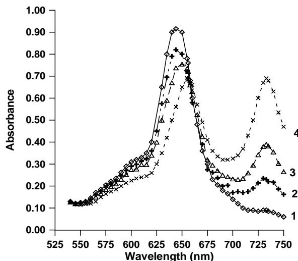
**Fig. 1.** Time dependence of the absorption spectrum for CHLA (19.0  $\mu\text{M}$ ). Measurements were made in time: 300 s (curve 1), half hour (curve 2), one hour (curve 3) and two hours (curve 4) after preparation of the solution
