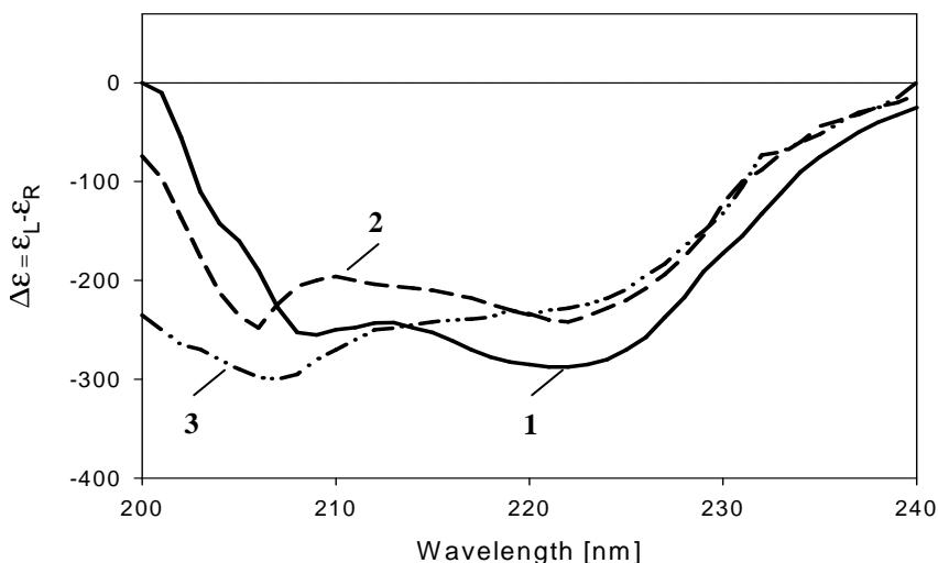
**Fig. 6.** UV- CD spectra of ferriCY (curve 1) and ferriCY with CHLA at the concentration of 0.3  $\mu\text{M}$  (curve 2) and 1.3  $\mu\text{M}$  (curve 3)
