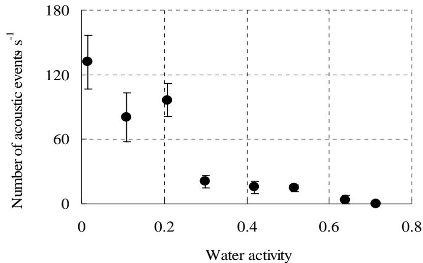
**Fig. 8.** Relationship between water activity and number of acoustic events generated during deformation of corn flakes
