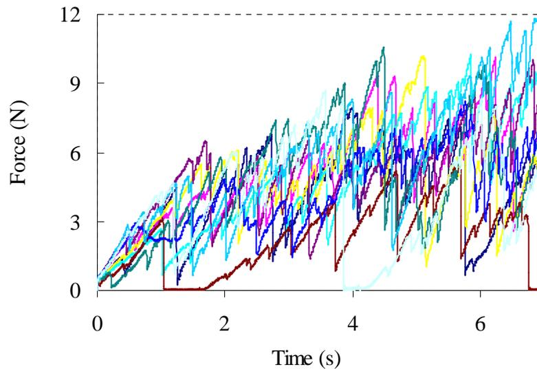
**Fig. 3.** Deformation curves for 10 samples of corn flakes  $a_w = 0.21$
