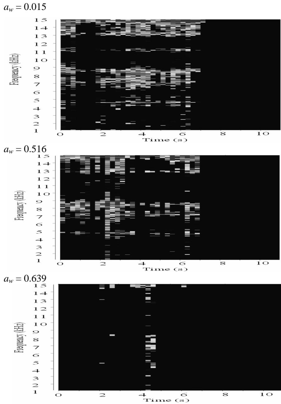
Fig. 7. Influence of water activity on acoustograms of corn flakes
