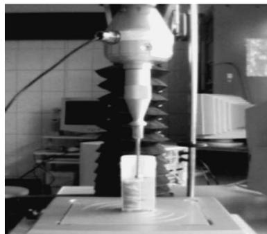
**Fig. 1.** Experimental stand for measurement of texture properties of corn flakes
