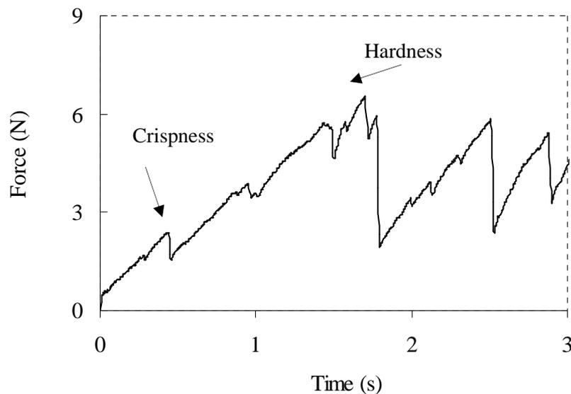
Fig. 2. Deformation curve of corn flakes at  $a_w = 0.21$
