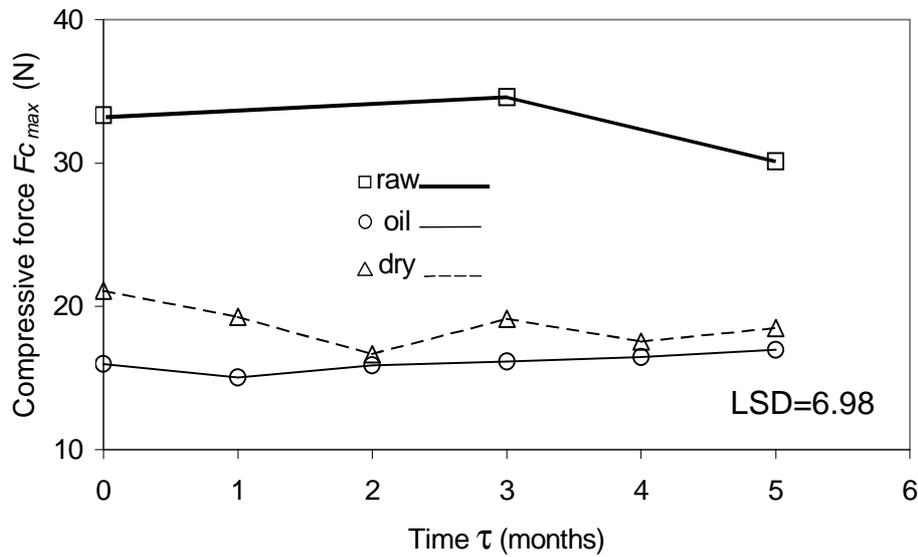
**Fig. 4.** Effect of storage time on maximum compressive force of raw and roasted walnuts (LSD - least significant deference refers to roasted walnuts)
