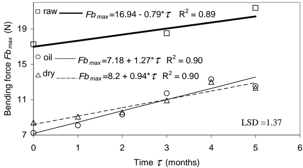
**Fig.3.** Effect of storage time on maximum bending force of raw and roasted walnuts (LSD - least significant deference refers to roasted walnuts)
