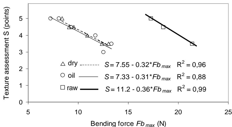
**Fig. 6.** Correlation between texture sensory assessment and maximum bending force of raw and roasted walnuts
