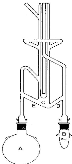
**Fig. 3.** Examining stand based on the Likens-Nickerson method
