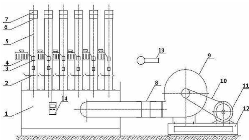
**Fig. 2.** Scheme of convection drying stand
