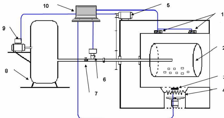
**Fig. 1.** Scheme of microwave-vacuum drying stand
