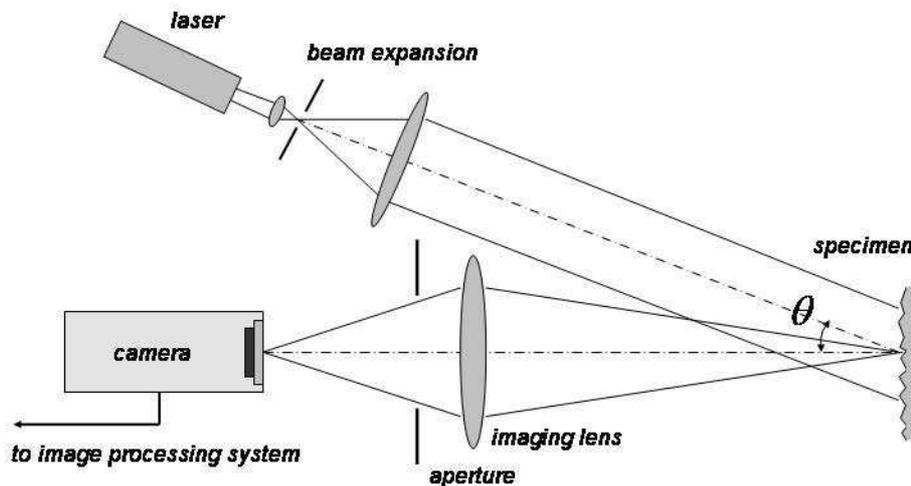
Fig. 1. Configuration of the system for spatial-temporal speckle correlation method
