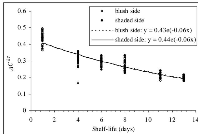
**Fig. 5.** Changes of the cross-correlation coefficient difference  $\Delta C^{k\tau}$  of apples during shelf-life for the blush and the shaded side
