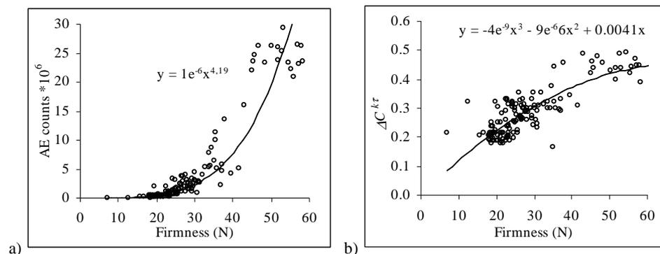
**Fig. 6.** Relationship between firmness and AE counts (a), and between firmness and the cross-correlation coefficient difference  $\Delta C^{k\tau}$
