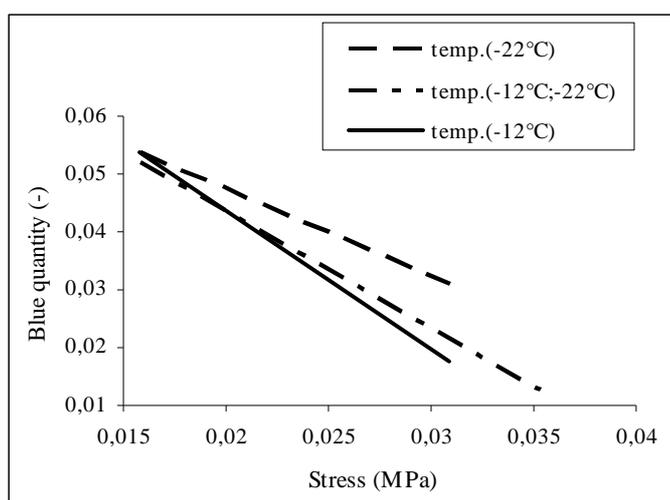
**Fig. 4.** Dependence of blue quantity changes from cake stress changes in a time function
