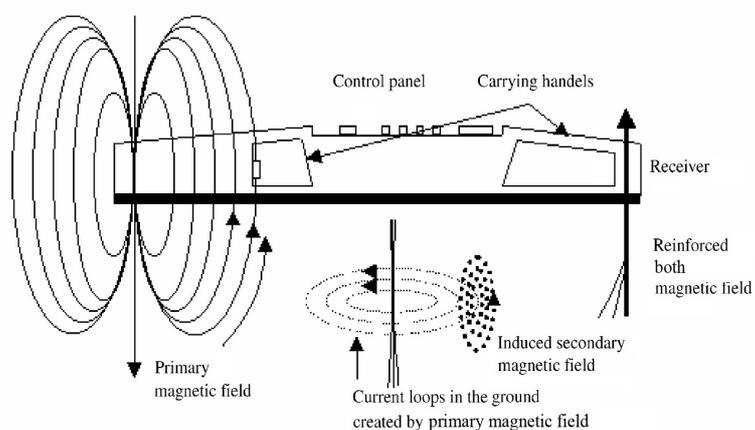
**Fig. 1.** Principle of EM-38 operation (Lesch *et al.* 2005, modified)
