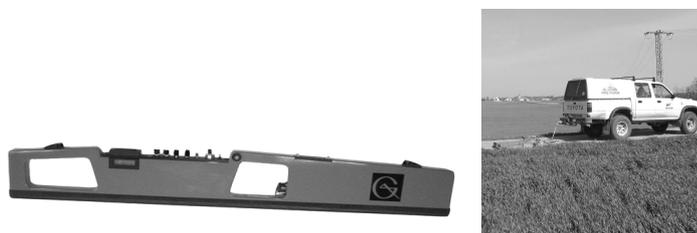
**Fig. 3.** EM-38 device and the off-road vehicle with EM-38 mounted on a wooden sledge
