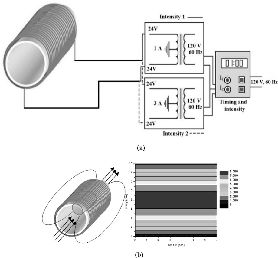
**Fig. 2.** Prototype irradiating of the electromagnetic field
