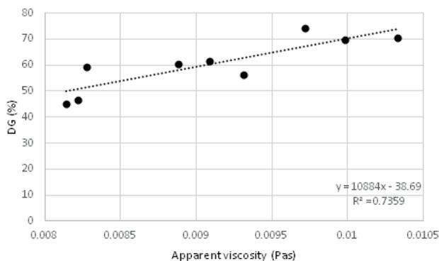
**Fig 2.** Correlation between apparent viscosity of pasta suspension (10% w/w) and degree of starch gelatinisation (DG)
