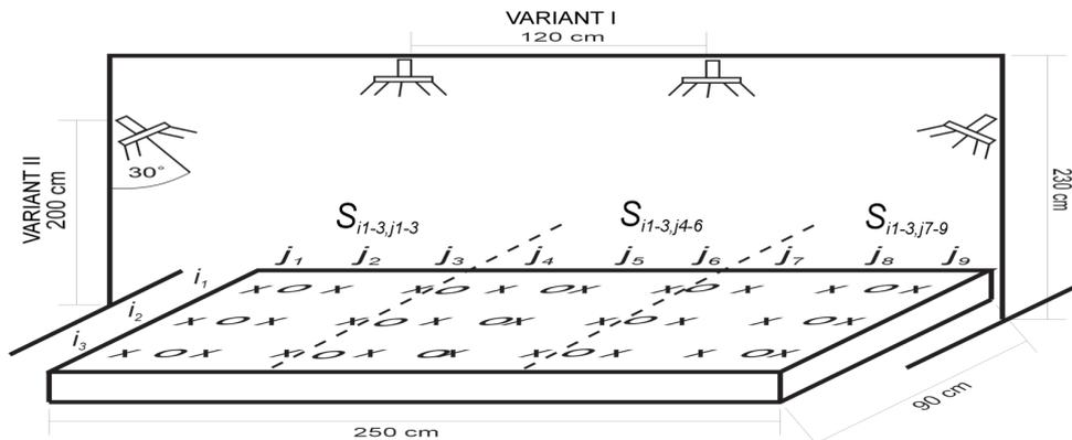
**Fig. 1.** Sensors (x = thermometers, o = thermocouples) location and IR heaters position in both variants of experiment (VARIANT I, VARIANT II) at the plot
