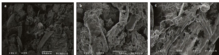
Fig. 1. Scanning electron micrographs of extrudates. Raw composition: 20% meat-bone pulp and 80% barley meal; barrel temperature profile: 120/140/180/180/130°C. Magnification: a) x35; b) x500; c) x1000
