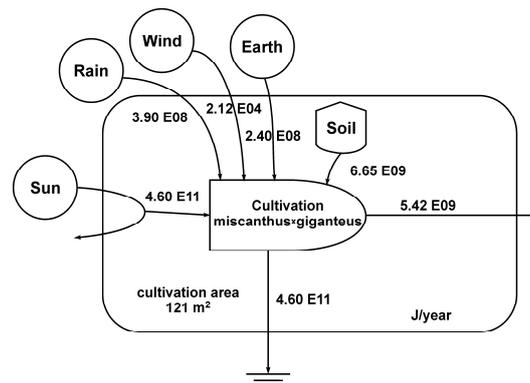
**Fig. 1.** Diagram of model cultivation of *miscanthus*×*giganteus* system located at the premises of University of Agriculture in Krakow, depicting energy flow to and from the system expressed in  $\text{J year}^{-1}$
