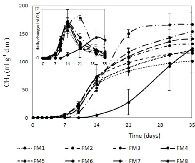
**Fig. 1.** Cumulative production of methane from tested samples in the function of time. The average of three replications  $\pm$  SD, inset: daily changes in  $\text{CH}_4$  production calculated for adjacent measurements. Explanations as in Table 3.
