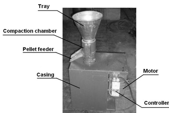
**Fig. 1.** Presentation of the pellet mill used in the study
