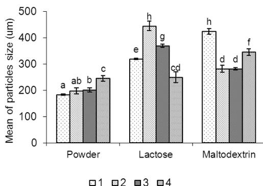
**Fig. 1.** Particle size of infant milk powder before and after agglomeration; 15% lactose solution and 20% maltodextrin solution were used as wetting liquids. The results are expressed as mean values with standard deviation. Values followed by a different letter are significantly different at  $p < 0.05$ .
