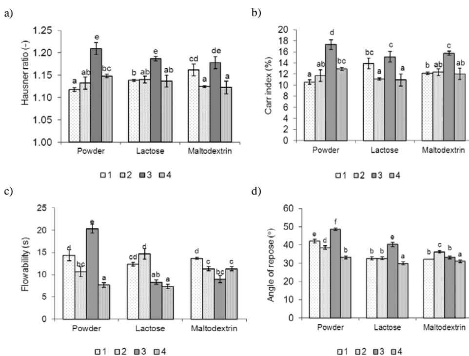
**Fig. 3.** Flowability factors of infant milk powder before and after agglomeration; 15% lactose solution and 20% maltodextrin solution were used as wetting liquids: a) Hausner ratio, b) Carr index, c) flowability, as pouring time, d) angle of repose. The results are expressed as mean values with standard deviation. Values followed by a different letter are significantly different at  $p < 0.05$ .
