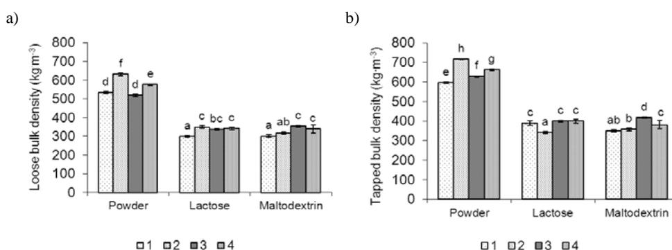
**Fig. 2.** Loose (a) and tapped (b) bulk density of infant milk powder before and after agglomeration; 15% lactose solution and 20% maltodextrin solution were used as wetting liquids. The results are expressed as mean values with standard deviation. Values followed by a different letter are significantly different at  $p < 0.05$ .
